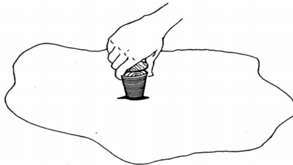
Installation of Wood Plug
